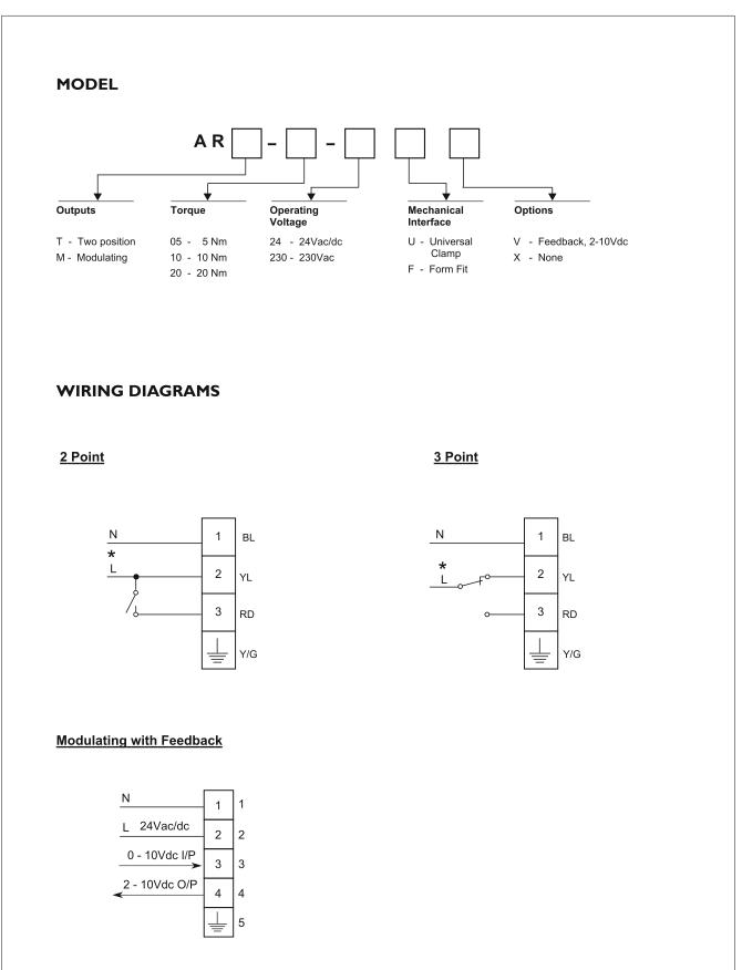
NOTE : \* 230Vac or 24Vac/dc depending on actuator working voltage.
